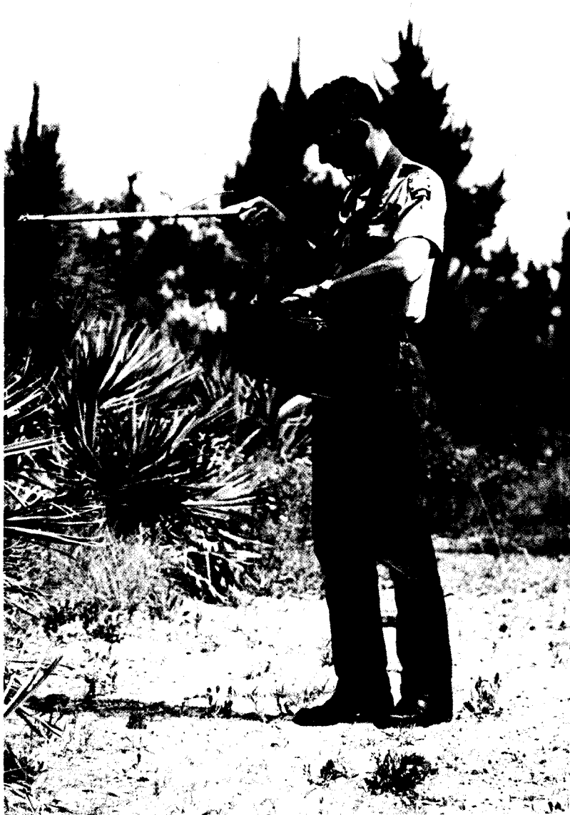
Figure 4. Receiver operator, with hand-held antenna, adjusting dials on receiver for accurate bearing.
