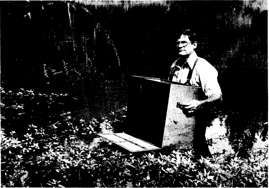
Figure 1. Sampler in position over plant community, showing sliding door open.
