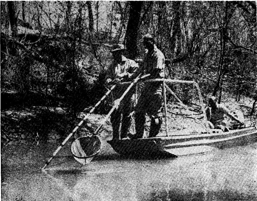
ALUMINUM ELECTRO FISHING BOAT IN OPERATION
