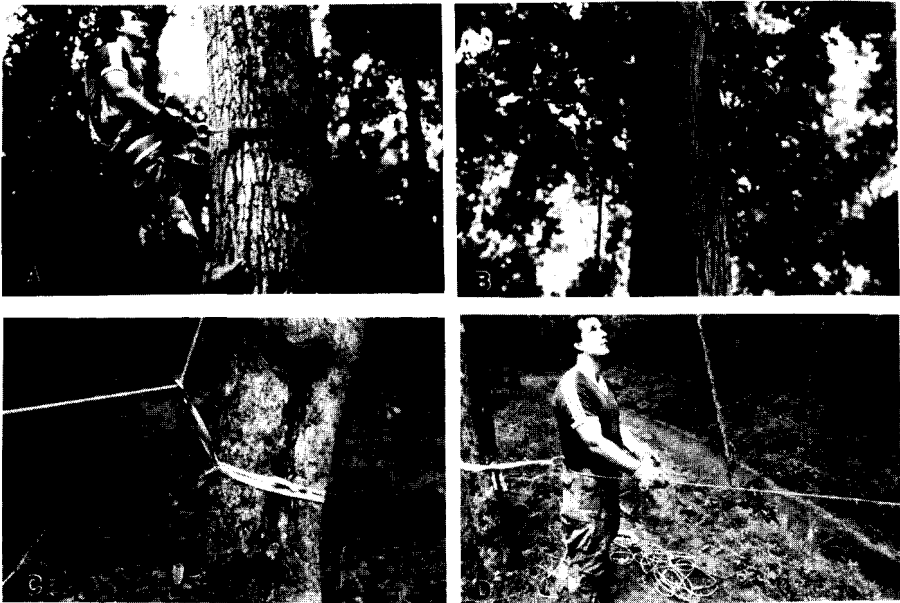
Figure 1. Equipment used in top rope climbing technique for cavity inspection: a tree pruner's saddle with pole strap (A), a climbing rope extended above a fork or branch above the cavity (B), a friction point on the climbing rope at ground level (C), and the body belay (D).
