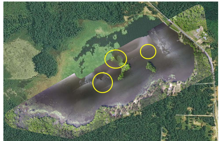
Figure 2. Bragg Lake, Ouachita County, Arkansas. Photogrammetric map from photos taken in April 2017 overlaid on Google Earth imagery from August 2014. Artifacts of poor photo alignment visible, such as smearing around the central island and banding on the lake surface identified by circle.
