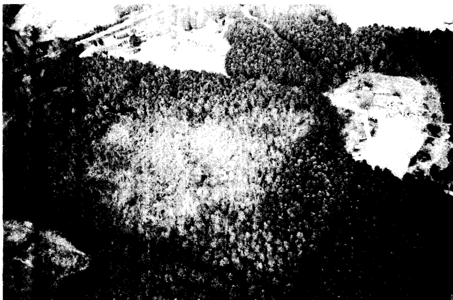
Figure 1. Black and white panchromatic photograph. Lighter tone within the pine stand represents area of heavy tree mortality.
