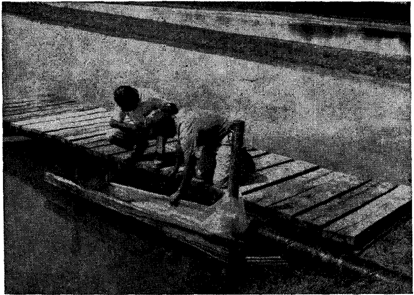
FIGURE 2.—THIS MONOFILAMENT FILTER SCREEN EFFECTIVELY PREVENTS TRASH FISH INTRODUCTIONS WHEN ATTACHED TO LOW VELOCITY DISCHARGE PIPES.
