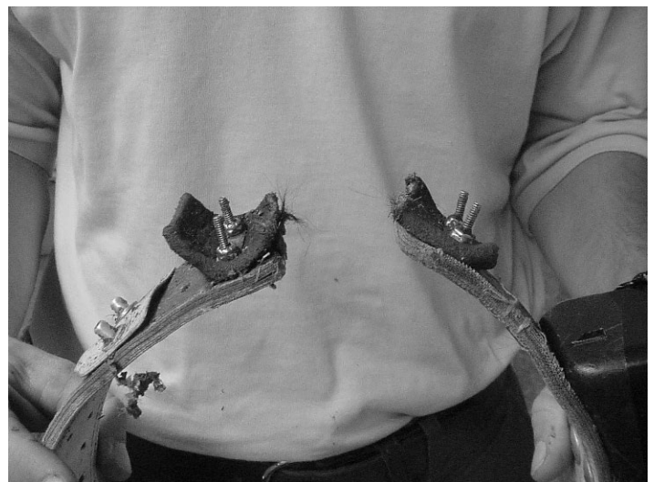
Figure 2. Radio collar dropped by a black bear with a broken leather spacer in Georgia.
